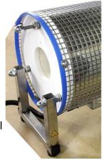
TMS Europe offers a range of control systems for use with our range of tensile test furnaces (used for creep test, stress rupture test, etc). Our standard 'MetTest' range provides precise and stable temperature control of 3 furnace zones. We can also provide bespoke solutions to meet your requirements, including phase-angle output, automatic 3-zone PID control, recording and LED bargraph power indicators.
