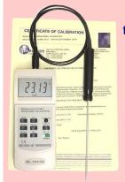
3mm probe reference thermometers with 0.01° resolution. With UKAS calibration at multiple points, including: -18, 0, 70, 100, 120, 165°C.
