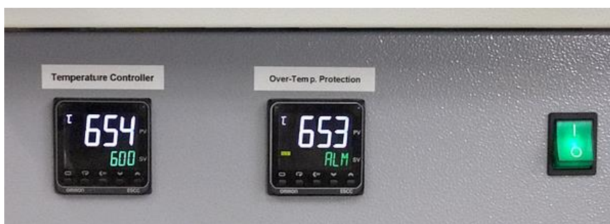
Optional OTP 2 and standard Temperature Controller. 'ALM' flashes on the display when over temperature.
