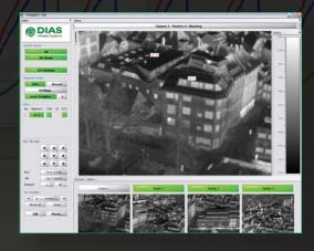
For fire detection: Use **PYROSOFT FDS** in combination with the intelligent early fire detection system PYROVIEW FDS to be able to react to fires in time. The cameras can be mounted on a pan-tilt head and thus cover the surveillance area in consecutive sectors.
