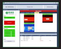
For a better overview: Use **PYROSOFT Automation MC** if you want to keep an eye on up to 8 different cameras at the same time. The data acquisition and analysis is done in parallel and independent from the other cameras. It is also possible to combine the measurements from different cameras for evaluation.
