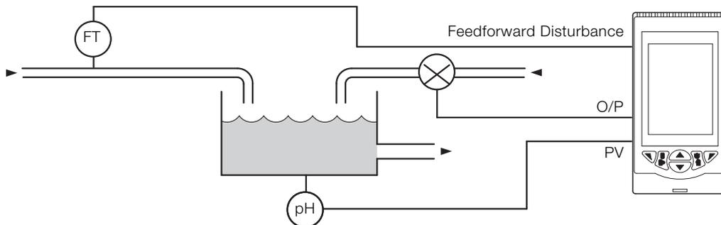
Fig. 20: Single loop with feed-forward
