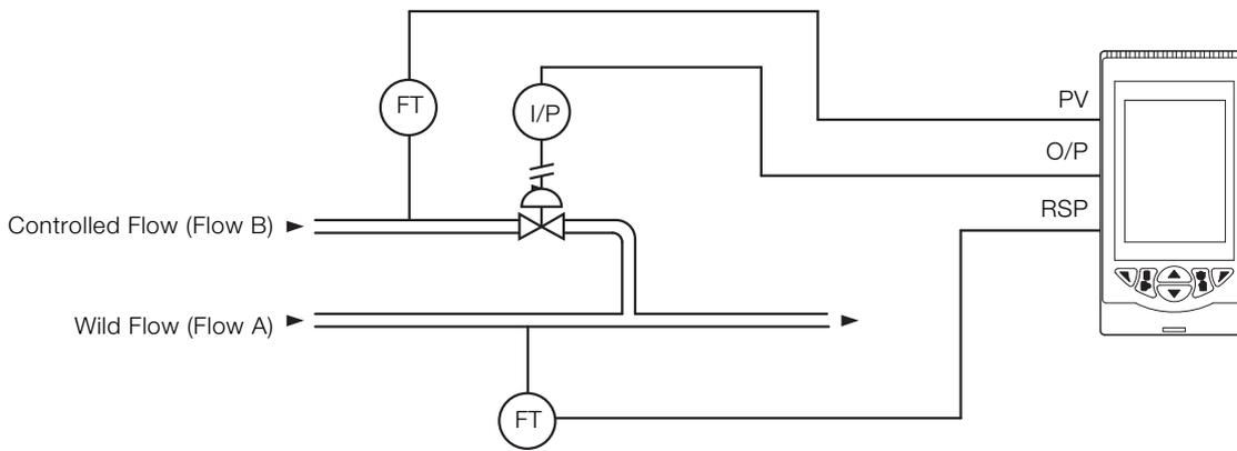
Fig. 23: Ratio controller
