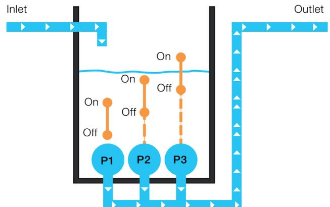
Fig. 13: Independent on and off trip points
