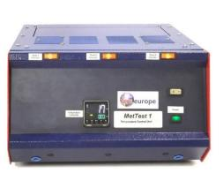
**Output Method:** Time proportioned Solid State Relay. Protection method: Relay controlled by main controller to protect against SSR failing on. **Over-current protection:** Fuse for each zone and system fuse. (No circuit breaker.) **Power Output:** 12.5A / 3kW max Power Connection: UK (BS1363) 13A plug (16A option available) Thermocouple Sockets: Type N as standard (additional options available)
