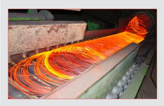
"metallurgical production a burning hot metal is stretched out through rollers" Copyright Andriy Solovyov , 2012 used under licence from Shutterstock.de
