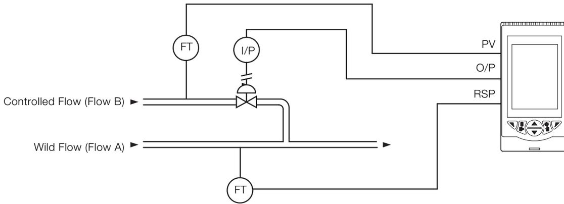
Fig. 23: Ratio controller
