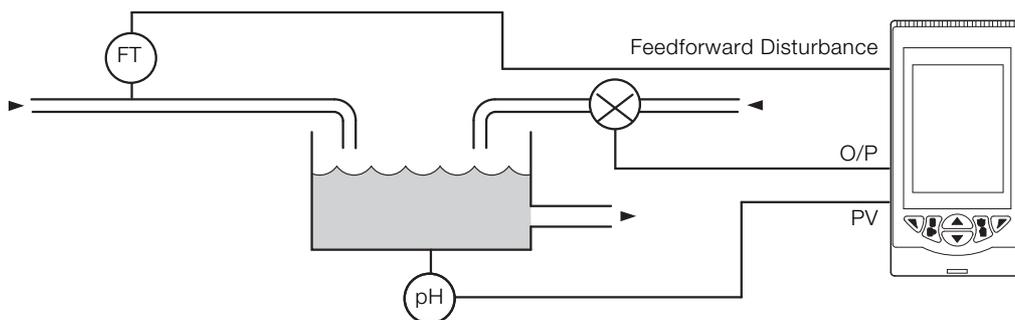
Fig. 20: Single loop with feed-forward
