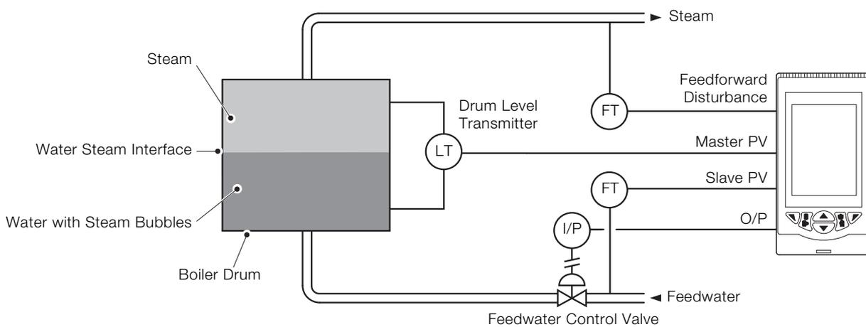
Fig. 22: Cascade with feed-forward
