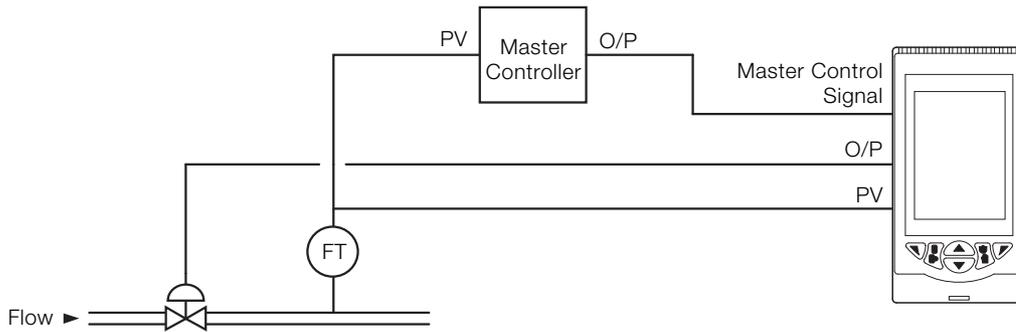
Fig. 25: Auto / Manual station and analog backup station
